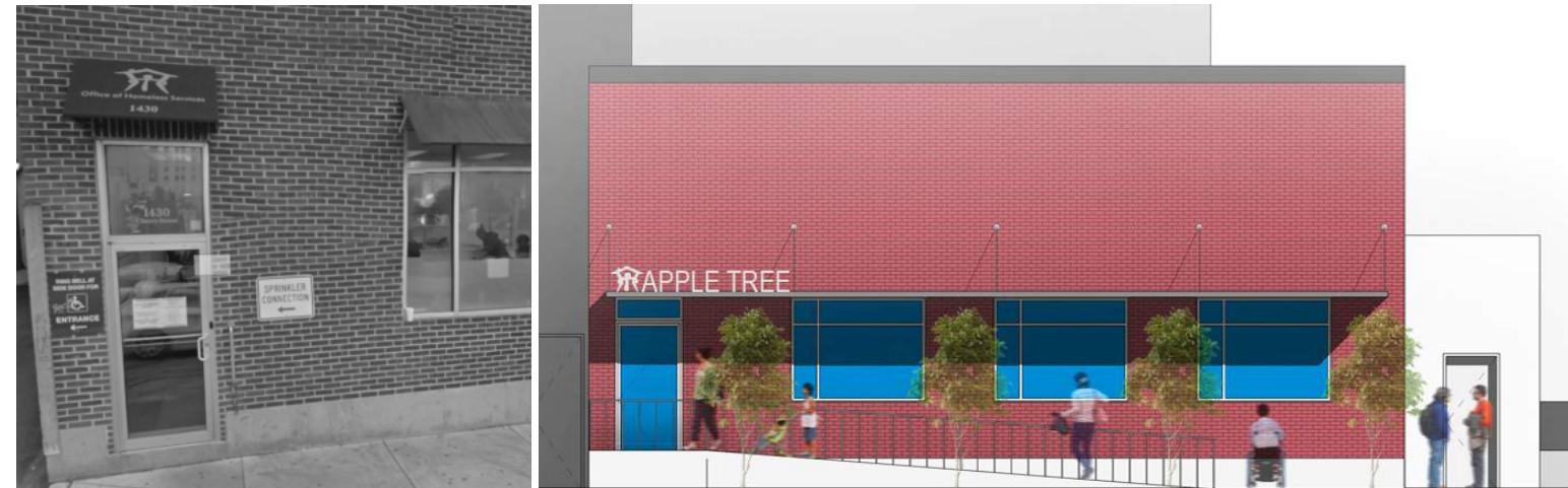
Before / Proposed redesign: Accessible entryway with a ramp ensures all participants enter and exit the site the same way.
